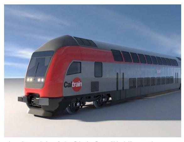
An artists rendering of what Caltrains fleet will look like once the commuter rail system switches from diesel to electric power. The trains, dubbed electric multiple units, or EMUs, will connect to wires running above the tracks. Caltrain estimates the electrification project will be finished by 2020. (Courtesy of Caltrain)
